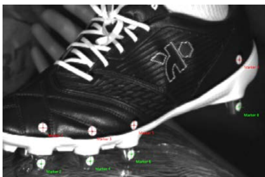
Figure 1: Eight shoe markers were used to obtain foot speed.
